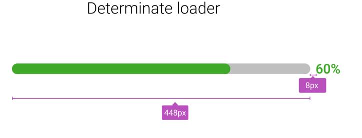
• Determinate progress indicators fill from 0 to 100%. • A percentage indicator appears as the progress indicator fills.
